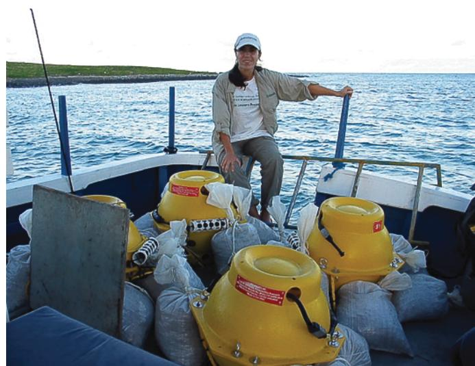
**Figure 3.** “Pop-ups”—marine autonomous recording units developed by the Bioacoustics Research Program at Cornell University—are ready to be deployed at sea.
